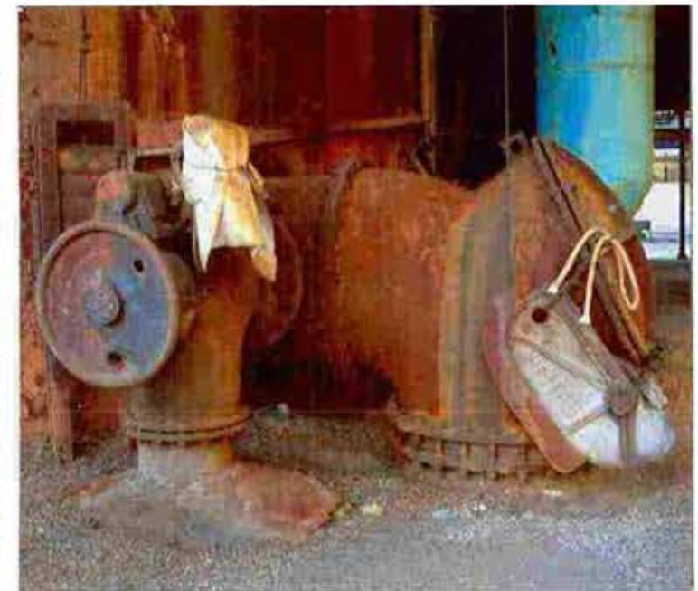
Cross-section of the Blast Furnace "A" compound according to the technical dossier dated 1967 and the photos of the stack valves, cut-off valves and the intake sections of the cold blast pipelines at the heaters.
